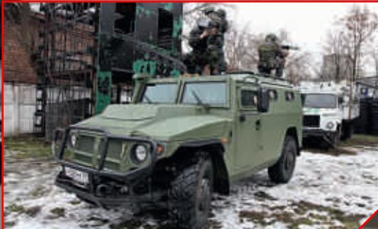
**SBM VPK-233136 TIGR special armoured vehicle is designed for carriage of troops and cargo on general-purpose roads and in rugged terrain, for use as a means of transport and a service vehicle of police forces on counterterrorist operations and riot control operations.**
