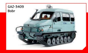
in the Far North, Siberia and Far East regions. The vehicles are designed for outdoor storage and operation in temperatures ranging from -50°C to +50°C in various road and climatic conditions and on any surface with a low load-bearing capacity — on snow, in sand, swamps and marshes — as well as for crossing water. Waterborne propulsion is provided by the tracks.
