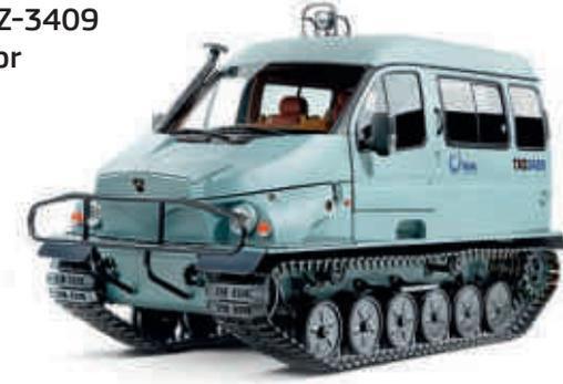
in the Far North, Siberia and Far East regions. The vehicles are designed for outdoor storage and operation in temperatures ranging from -50°C to +50°C in various road and climatic conditions and on any surface with a low load-bearing capacity — on snow, in sand, swamps and marshes — as well as for crossing water. Waterborne propulsion is provided by the tracks.
