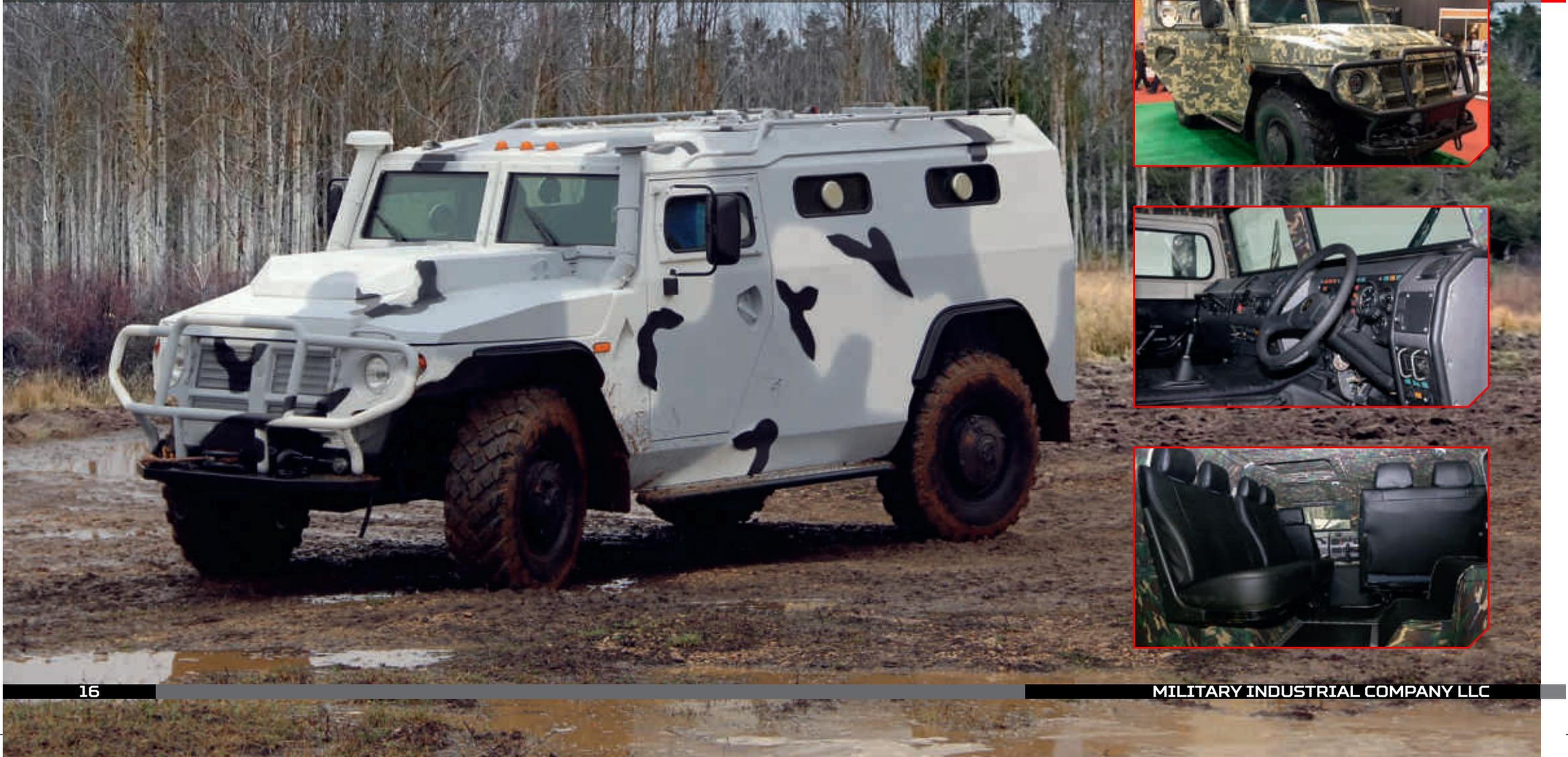
**SBM VPK-233136 TIGR special armoured vehicle with a right-hand drive is designed for carriage of troops and cargo on general-purpose roads and in rugged terrain, for use as a means of transport and a service vehicle of police forces on counterterrorist operations and riot control operations in countries where left-hand traffic is traditionally accepted.**
