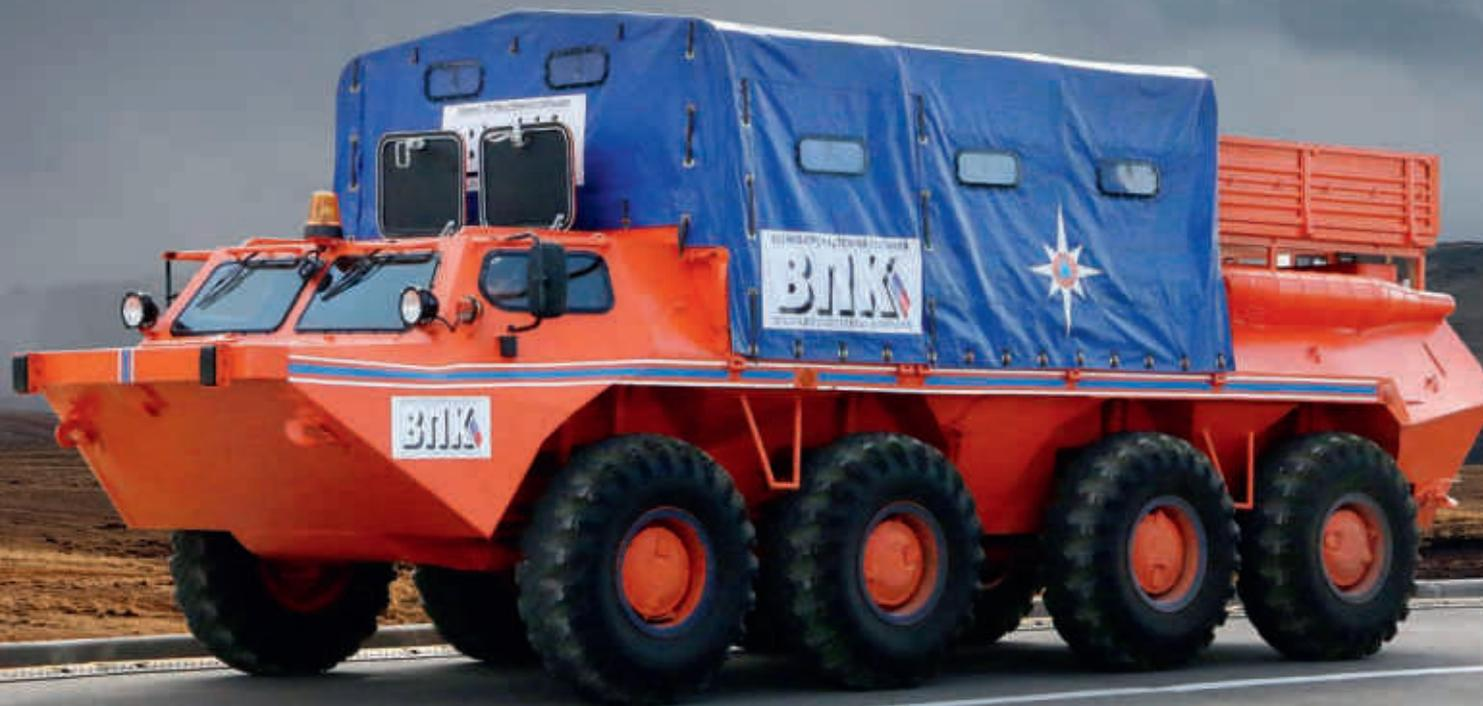
**59037 and 59037A all-terrain amphibious vehicles are designed to carry passengers and cargo on all kinds of roads, as well as off-roads with a possibility to cross the water barriers.**
