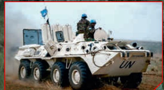
The BTR-80 APC is a fully amphibious combat wheeled vehicle designed to carry an infantry or marine squad and provide it fire support in battle and for the squad to fire from inside the vehicle as well.
