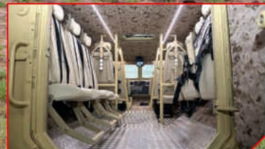
Developed by the staff of the Military Industrial Company at its discretion and expense, the 4 × 4 VPK-Ural armoured multipurpose vehicle is designed to carry troops and cargo, as well as tow trailers and mount weapons and special equipment providing the required protection level.
